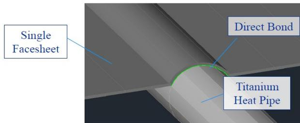
Figure 17. Single face sheet radiator with direct bonding of the face sheet to the heat pipes
