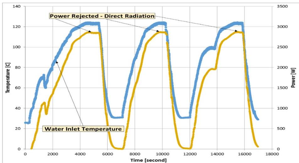
Figure 22. Power rejected in vacuum during the second round of testing when maximum inlet water temperature was 127°C.
