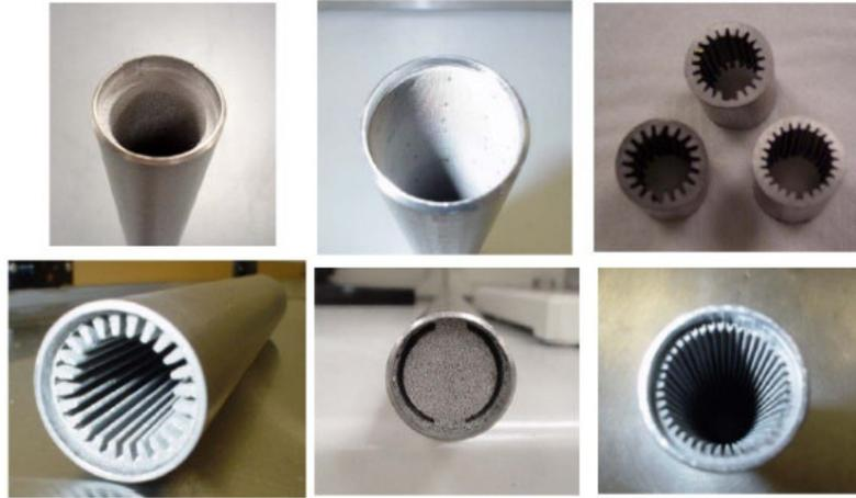
**Figure 6. Heat pipe wicks developed on the RDU program. Counter-clockwise from top right: (a) solid groove wick, (b) screen wick for life test pipes, (c) sintered annular wick for life test pipes, (d) sintered vapor-groove wick, (e) slab wick, and (f) sintered liquid groove wick.**
