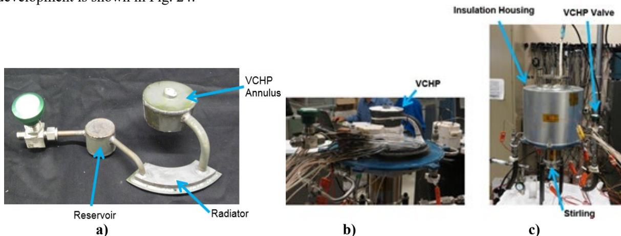
**Figure 24. Sodium VCHP as Backup Cooling System for Stirling RPS a) Actual prototype b) The prototype integrated with Stirling converter and c) VCHP and insulation housing installed on the Stirling converter and ready for testing at NASA GRC.**
