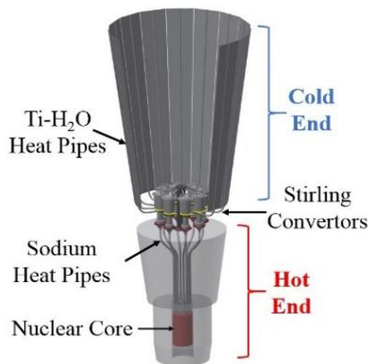
**Figure 7. Kilopower system conceptual design and its thermal management system [25].**
