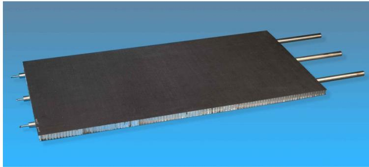
**Figure 5. Three RDU panels with Graphite Fiber Reinforced Composite (GFRC) face-sheets and titanium heat pipes were delivered to NASA Glenn for testing. Each panel was 1m by 0.5m, had three heat pipes, and was designed to operate at temperatures up to 550K.**
