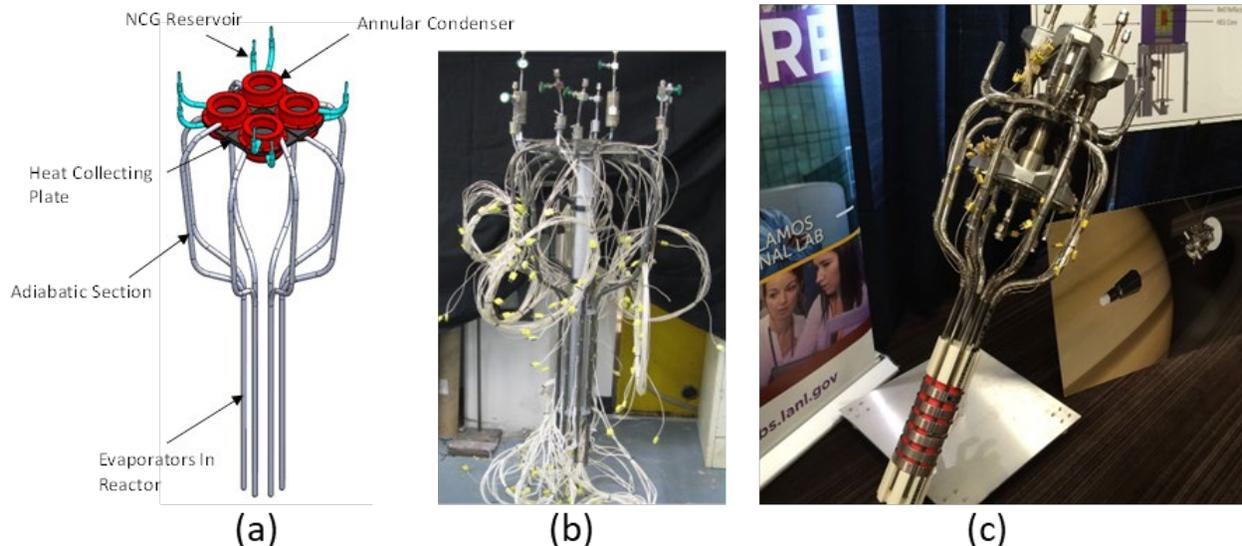
**Figure 8. Kilopower system: a) Schematic of the Kilopower heat pipes and heat collector plate. b) Thermosyphons (First Set) fabricated by ACT for the electrically heated Kilopower system c) Sodium heat pipes (Second Set) developed by ACT for Kilopower and displayed by NASA at NETS 2018.**
