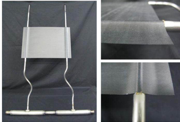
**Figure 18. Small-scale, proof of concept titanium/water radiator for Lunar fission power operations. The panel is directly bonded to the heat pipes, reducing mass.**
