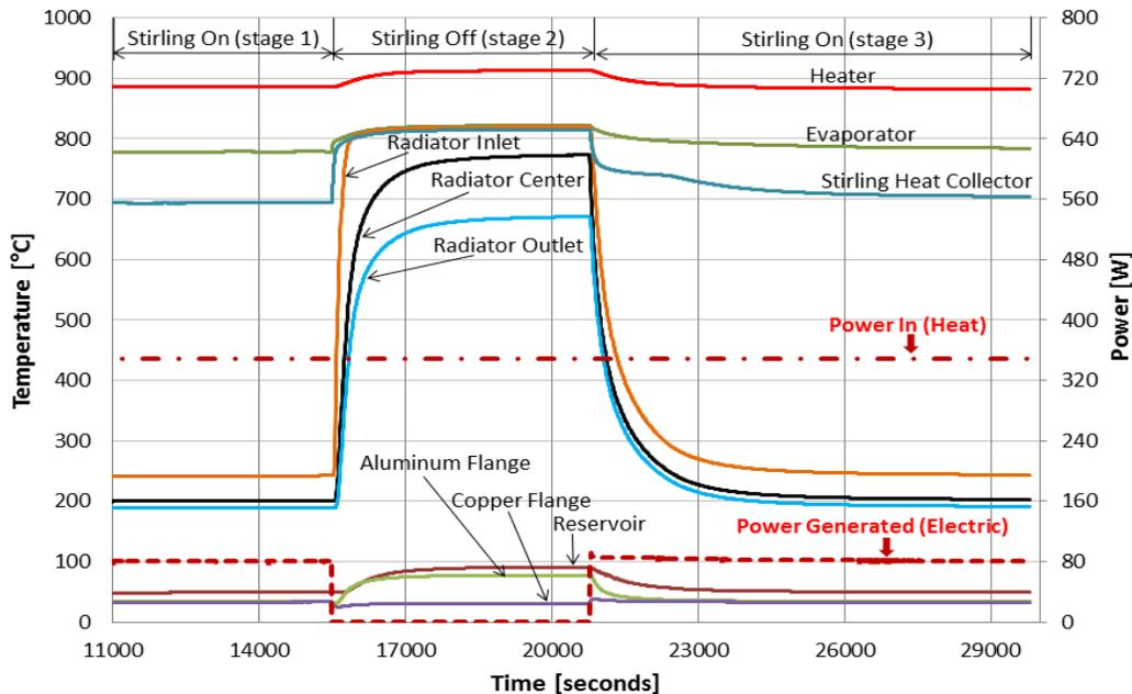
**Figure 25. Experimental results for the long duration stoppage test - steady state achieved each time.**
