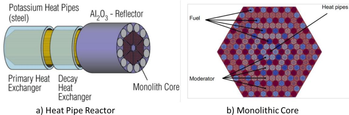
**Figure 1. Heat pipe reactor design proposed by LANL [2], b) Pattern of fuel rods and heat pipes in a heat pipe reactor's monolithic core [3].**
