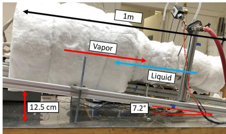
**Figure 23. Prototype high-power sodium heat pipe capable of transporting 2kW over 1m at an angle of 7° against gravity.**
