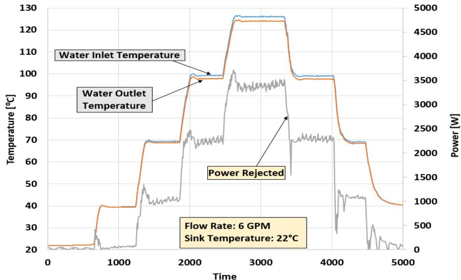
**Figure 20. Power test in ambient conditions at ACT: heat was rejected for various water inlet temperatures.**
