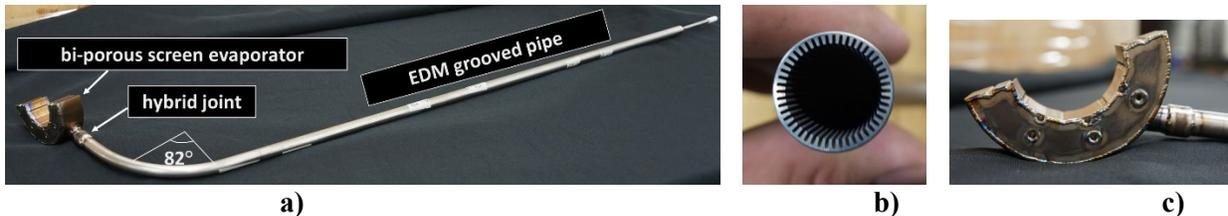
**Figure 12 a) Titanium water heat pipe with bi-porous screen evaporator and hybrid wick for the rest of the pipe. b) Grooved wick manufactured by electrical discharge machining (EDM). c) Evaporator section of the heat pipe that has a semi-circular shape to be mounted on the cold end of the Stirling converter.**
