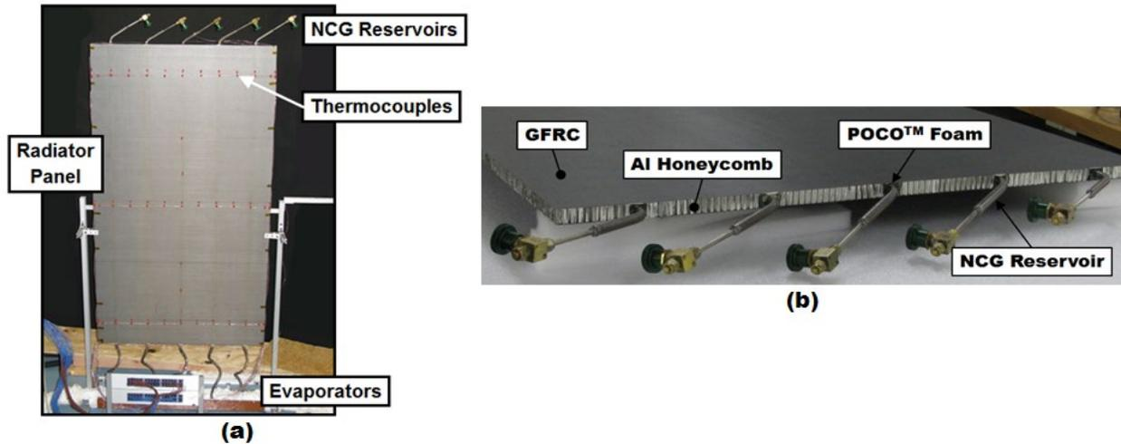
Figure 16. (a) VCHP radiator in testing configuration, (b) cross section of VCHP radiator.
