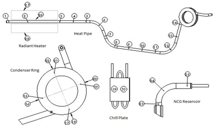
**Figure 11. Instrumentation layout of alkali metal Kilopower heat pipes.**
