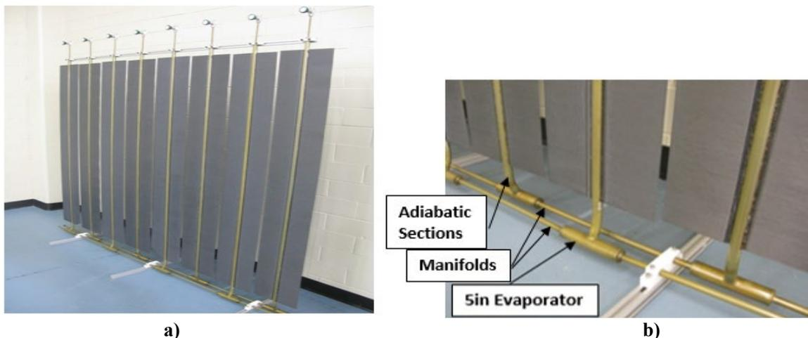
**Figure 19. First cluster a) Actual radiator cluster b) Detail showing the manifolds, the heat pipe evaporators and adiabatic sections.**
