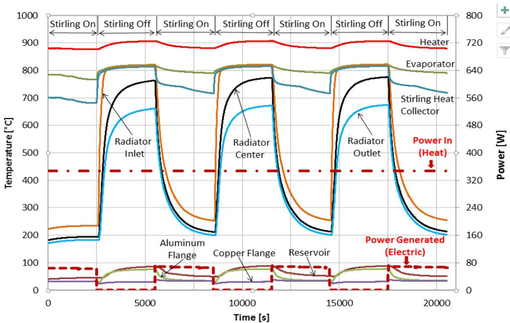
Figure 26. Experimental results for the multiple short duration stoppages testing of the Stirling converter with VCHP.
