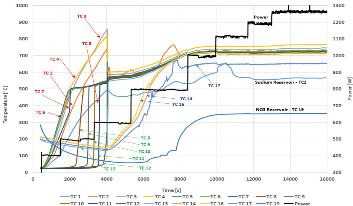
**Figure 9. Startup results for the First Set (generation) of thermosyphons.**
