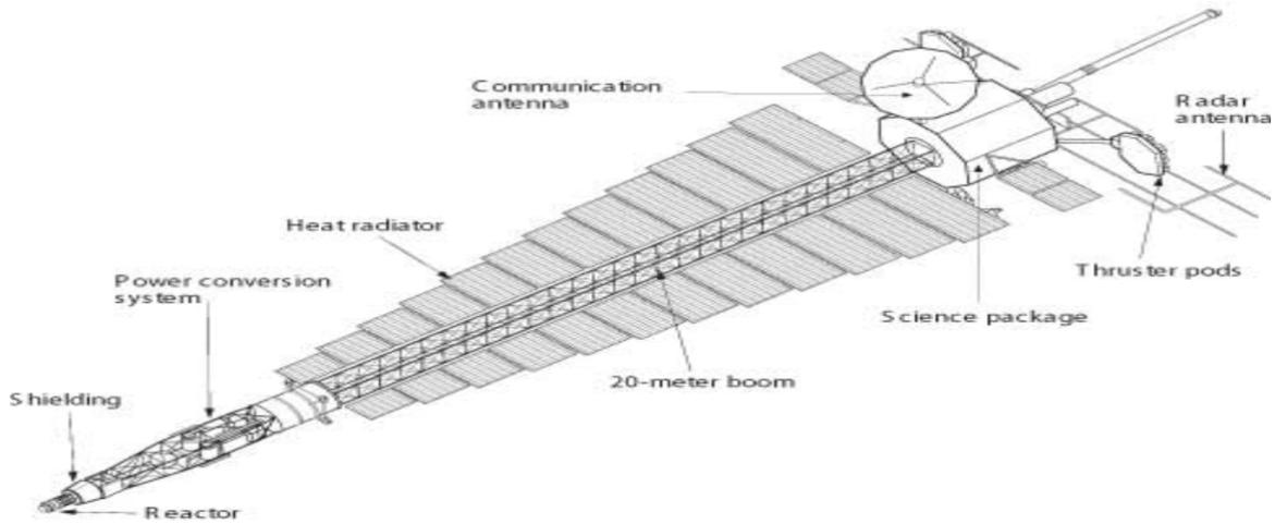
**Figure 4. JIMO conceptual design with a system of deployable radiator panels for heat rejection.**
