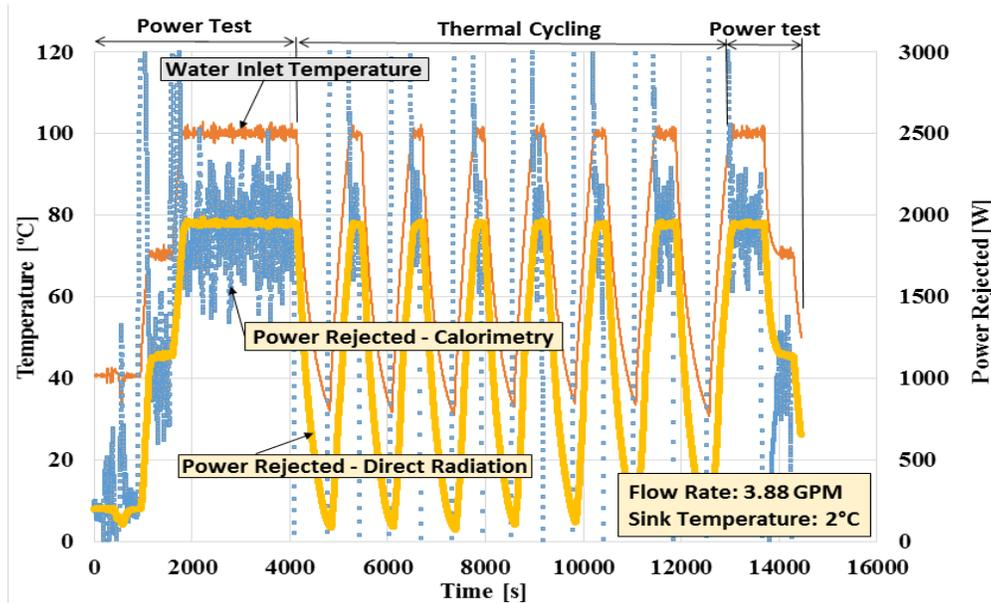
Figure 21. Radiator cluster testing in vacuum at GRC– first round: testing was carried out as power test, thermocycling and power test again.
