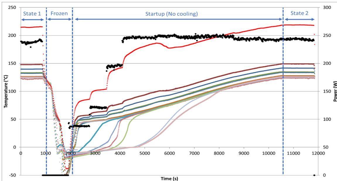
**Figure 13. Freeze/thaw startup performance of the titanium water heat pipe.**
