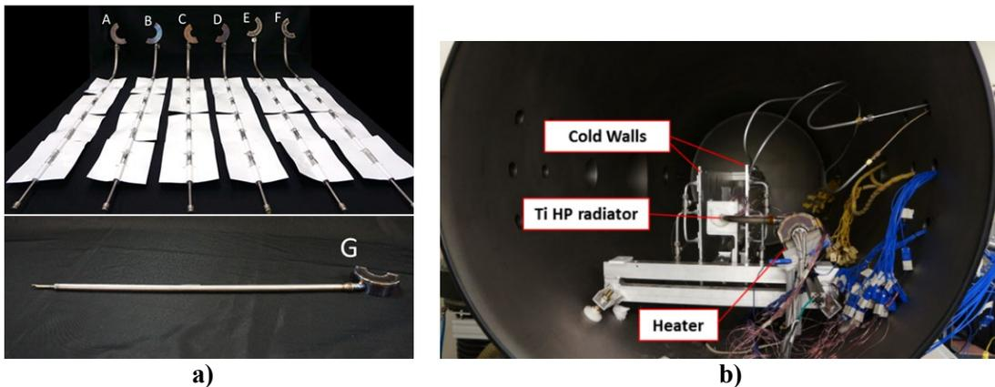
**Figure 14. a) Titanium water heat pipes for Kilopower system cooling (top: six full-length heat pipes with S-bonded radiator; bottom: half-length heat pipe for shock and vibration testing) b) Heat pipe radiator thermal performance test setup.**
