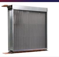
The Air-to-Air Heat Pipe Heat Exchanger (AAHX) uses the air exiting the building (cool in the summer, warm in winter) to either pre-cool or pre-heat incoming outside air.
