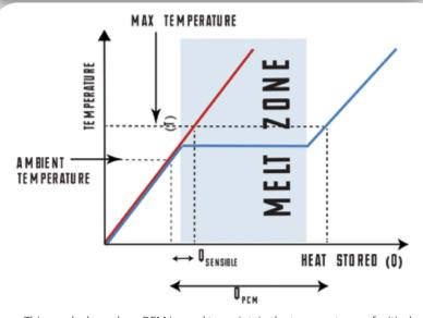
This graph shows how PCM is used to maintain the temperatures of critical heat-generating components over a given period of time.
