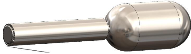
Figure 11: CAD model of the Lunar evaporator and compensation chamber.
