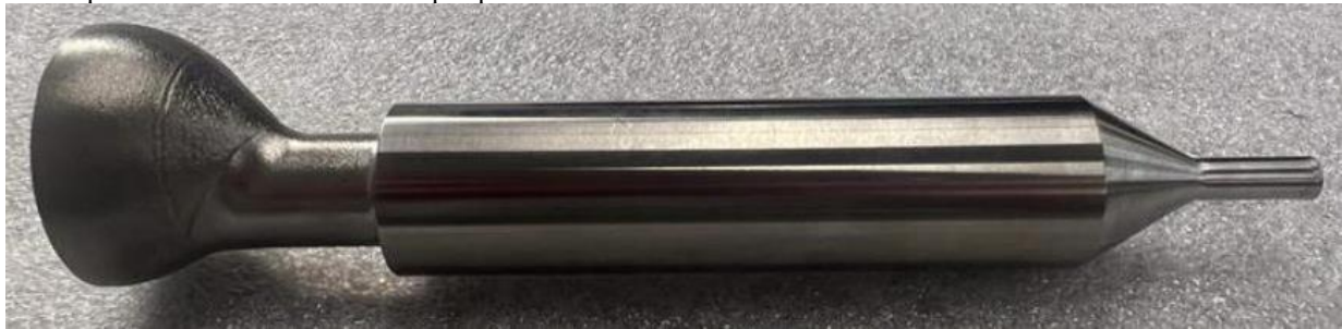
Figure 4: 3D-printed SmallSat evaporator. Note that the vapor plenum and the first half of the compensation chamber are included in the print.
