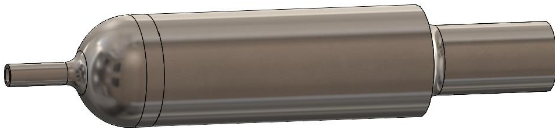
Figure 3: CubeSat Evaporator (CAD). Note that the vapor plenum is integrated into the print.
