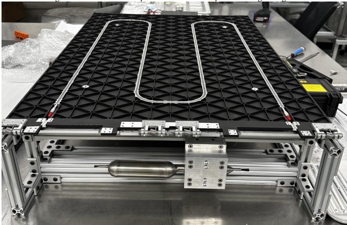
Figure 5: The assembled SmallSat deployable radiator panel, along with the pump body.
